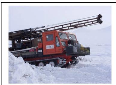
conduct its winter program. The drill is a hollow stem auger for collecting soil and rock core samples, and measuring soil strength at depth.
